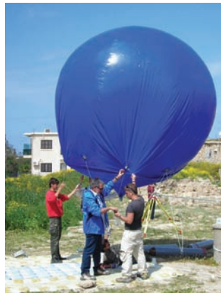
STARC, in collaboration with the Univ. of Sydney, CNR-ITABC, and the Univ. of Naples, set-up a balloon-suspended set of digital cameras – to produce a 3D model of a Hellenistic-Roman theater in Pafos (left).
